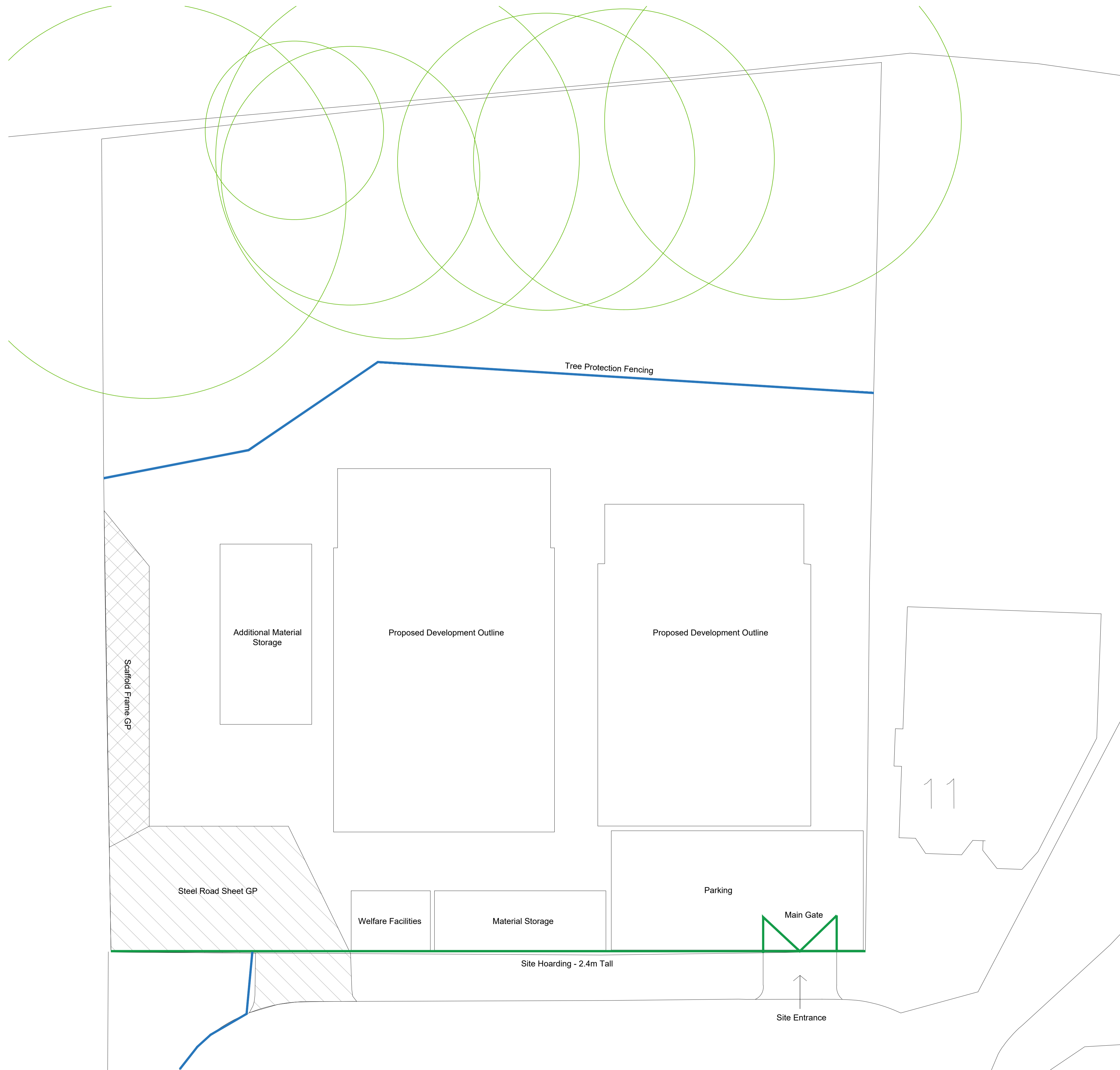
PROPOSED SITE LAYOUT DURING CONSTRUCTION - 1:100
